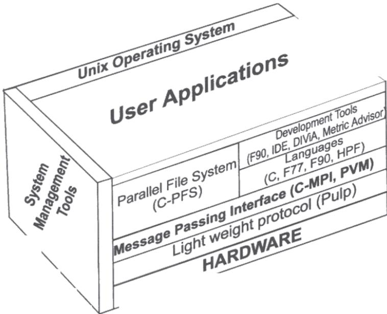
Figure 2: HPCC Software Architecture
